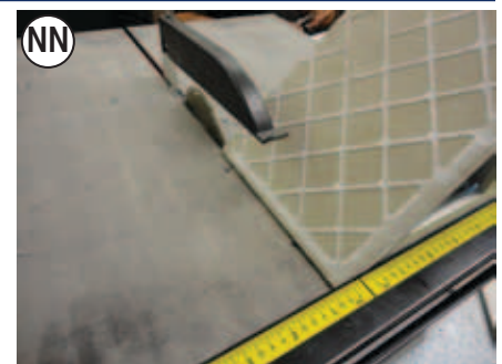
Figure NN: 45° Mitre Cutting using the Magnetic Angels.
