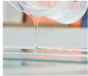
SilGel® 612 can be cast therefore particularly easy to process
