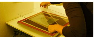
Place a clear glass over the foil, it must be big as the screen and it must press the foil completely to the screen.
