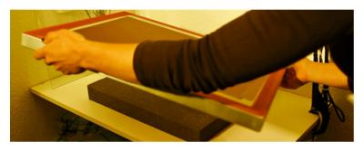
The styropor has to be in a size that will fit the inner frame and must be so thick that the screen lays directly and strong to it!
